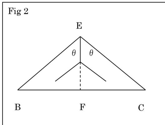
$$CF = \frac{BC}{2} = \frac{\sqrt{2}}{2}L \quad EF = \sqrt{\left(\frac{\sqrt{3}}{2}L\right)^2 - \left(\frac{\sqrt{2}}{2}L\right)^2} = \frac{L}{2} \quad \frac{1}{\tan \theta} = \frac{EF}{CF} = \frac{1}{\sqrt{2}} = \frac{\sqrt{2}}{2} \doteq 0.707$$
